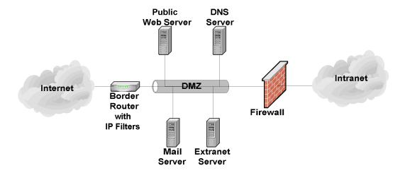
Figure 7.1: Simple Single Firewall DMZ
