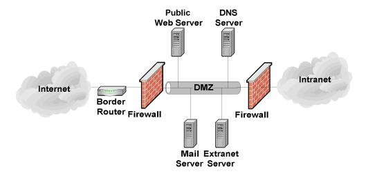
Figure 7.2: Two Firewall DMZ
