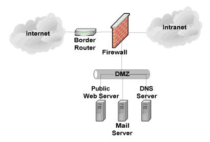
Figure 7.3: Three Interface Firewall DMZ
