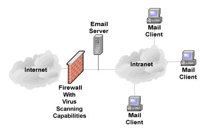
Figure 6.1: Virus Scanning Implemented on Firewall
